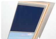
OptiLight VK window is equipped with manually operated air inlet positioned in the top part of the frame. It provides fresh air up to 19m<sup>3</sup>/h (at a pressure difference of 10Pa) when the window is closed.
