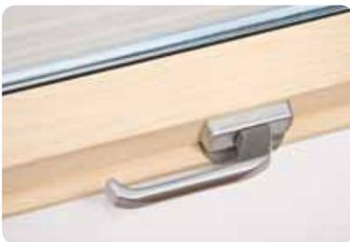
*The window is closed with the use of the handle positioned at the lower part of the sash. It allows locking the window at three points: closed tightly and two micro-opening positions.*
